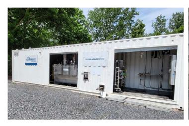
**PORTABLE LIME SLURRY – PRODUCTION**Fully Autonomous Slaking Solution
